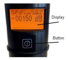
After first pushing of button from switched off display status is shown intro screen. There is shown basic information about probe as is version of firmware, serial number and status measurement running ON/OFF.
